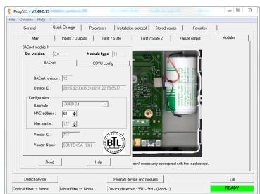
Note: The BACnet MS/TP module is compatible with Supercal / Superstatic integrators with firmware release FW 3.7 or higher (FW ≥ V3.7).
