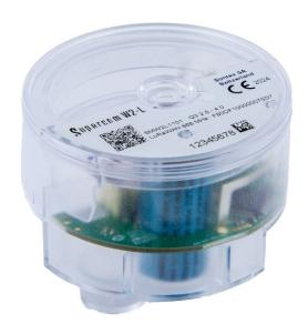
The radio modules of the *Supercom W2* (SMW2) family are adapted to Honeywell (Elster) Picoflux water meters with flow rates from Q3 2.5 m3/h to 4 m3/h. The water meters can be retrofitted at any time.
