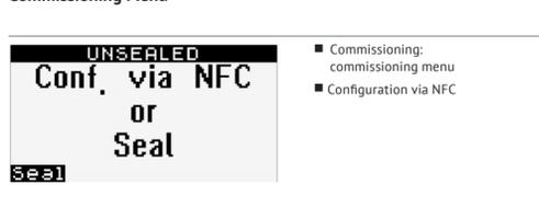
The sealing can be performed via NFC with the Superprog Android application or via optical head or M-Bus with the Superprog Windows application.
