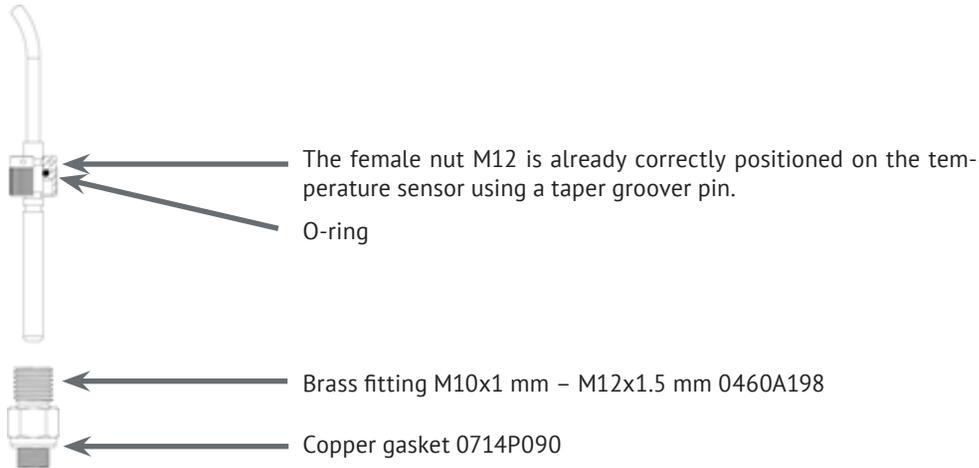
1. Place the copper gasket (0714P090) on the brass fitting M10x1 mm side.
