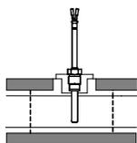
Insulation will only be provided as far as the fixing screw
