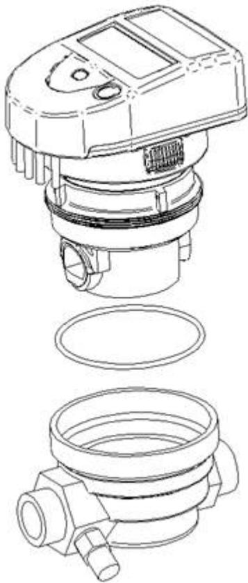
To mount the Supercal 739 coaxial multi jet with M77x1.5 connection in the EAS base, the following steps must be respected:
