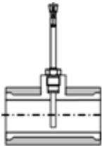
The temperature sensor is on the same level and perpendicular to the pipe axis (DN15, DN20)
