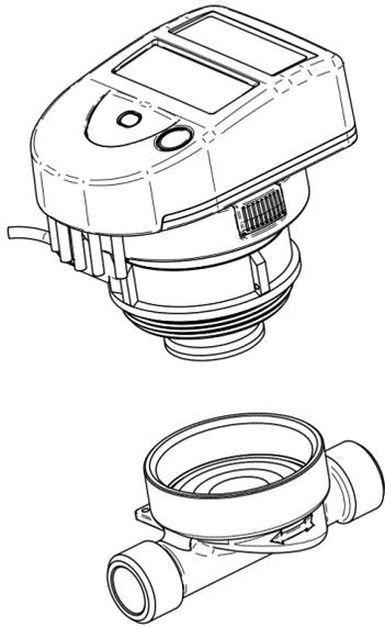
To install the Supercal 739 with coaxial multi jet with the M62x2 connection in the EAS base, the following steps must be respected:
