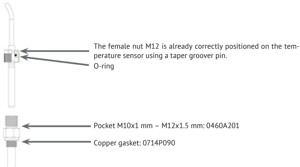
1. Place the copper gasket (0714P090) on the pocket M10x1 mm side.
