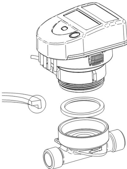
To install the Supercal 739 with coaxial multi jet with the G2" connection in the EAS base, the following steps must be respected:
