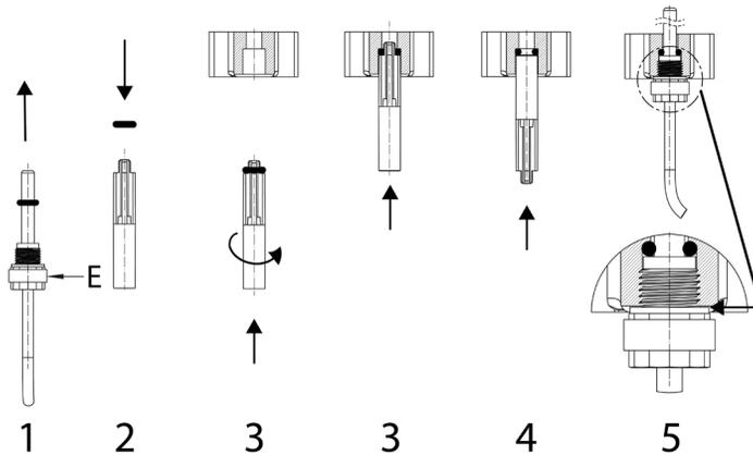
1. Remove the O-ring from the temperature sensor. Be careful not to remove the rubber band (symbolized by the letter "E" on the drawing) from the nut as it may separate into two parts and fall on the floor.
