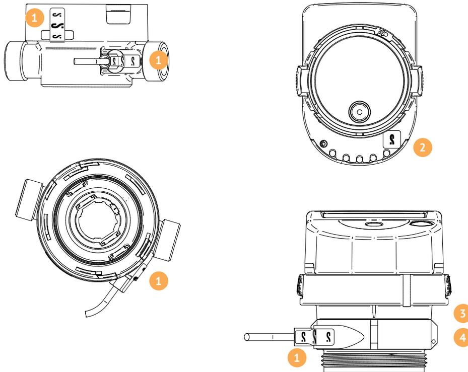
1 Seals installed in the factory on flow meter and temperature sensor of the Supercal 739
