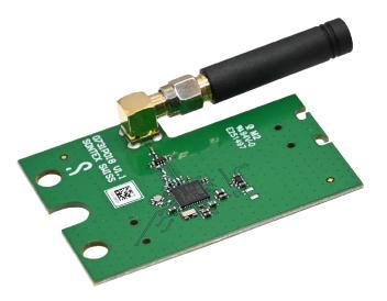
The LoRaWAN<sup>®</sup> certified radio communication module is used in combination with the thermal energy meter *Supercal 5 S* or the calculator *Supercal 5 I* in order to transmit the measured data over any private or public LoRaWAN<sup>®</sup> network. The payload contained in the long and short LoRaWAN<sup>®</sup> telegram is freely configurable. The status of the LoRaWAN<sup>®</sup> network connection is indicated on the display of the *Supercal 5 S/I*.
